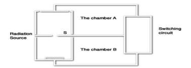
Fig III:-Working of Ionization smoke Detector
