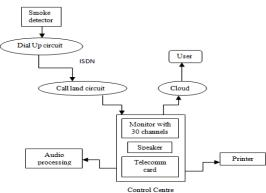
Fig I: Block Diagram of the System
